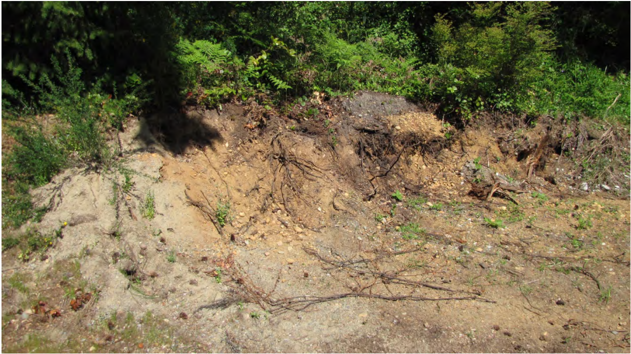
Photo. 1 Exposed sands and gravel – typical of the type found in the test well area.
