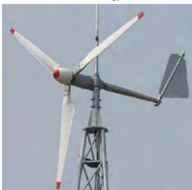
Horizontal axis turbine.
