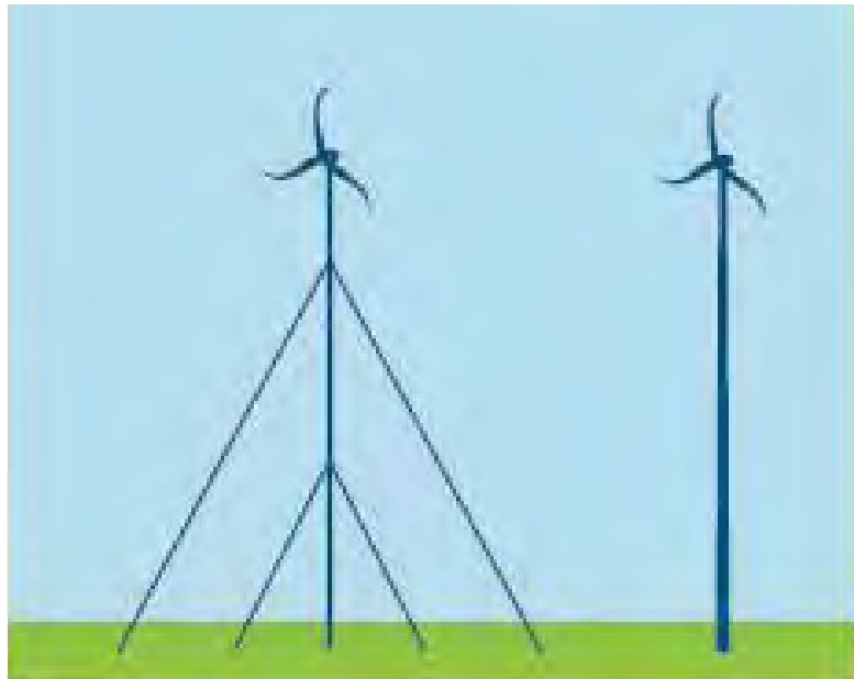
Guyed tower and monopole tower.
