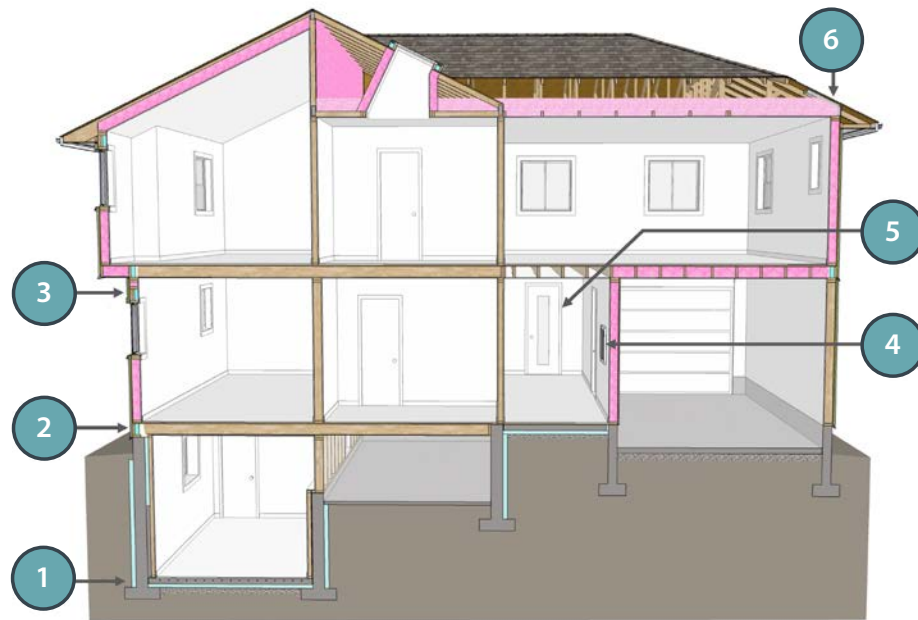
Figure 2: Typical Problem Areas for Insulation Continuity
