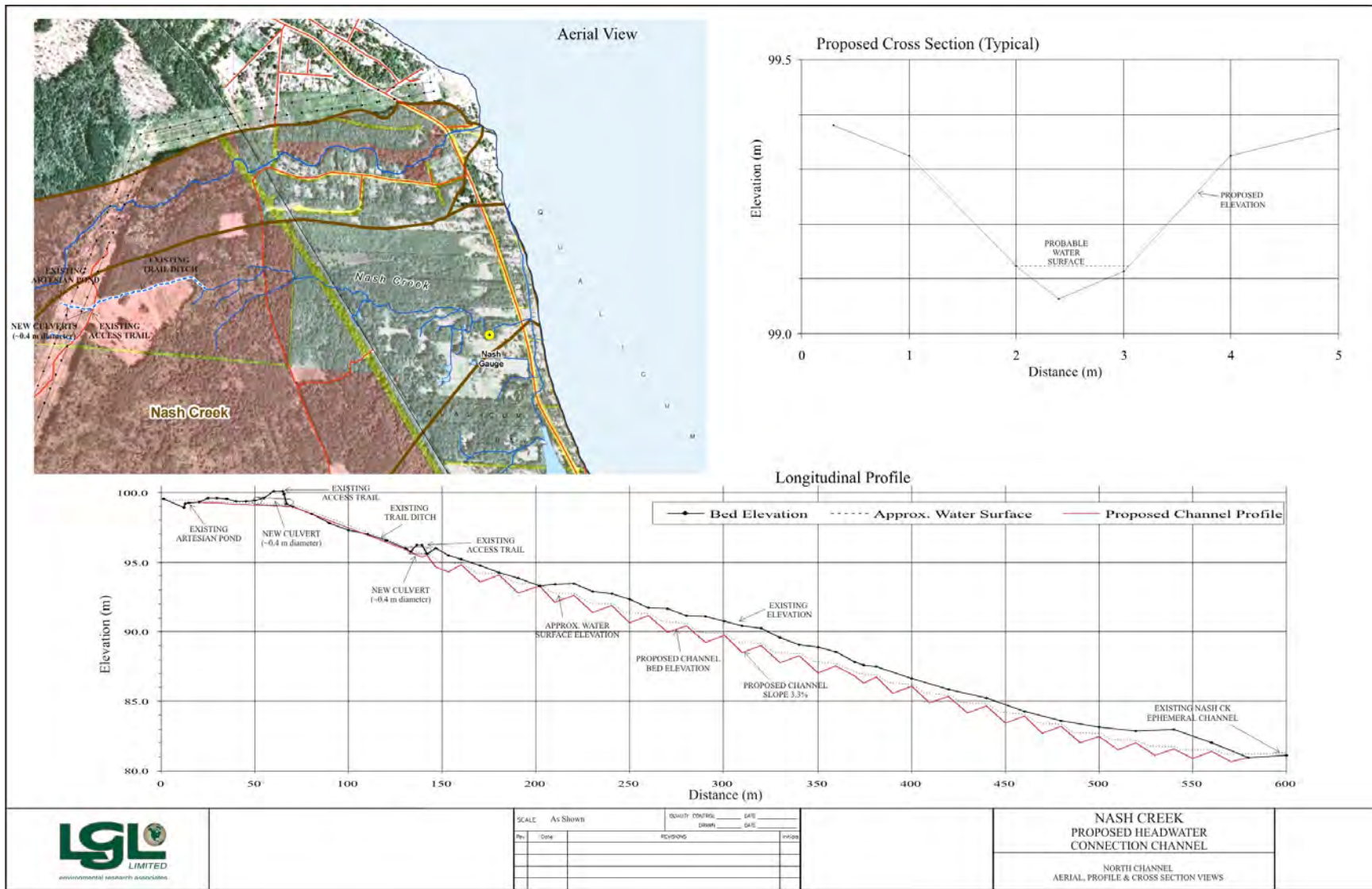
Figure 23. Conceptual drawing of headwater drainage network re-connection on Nash Creek.
