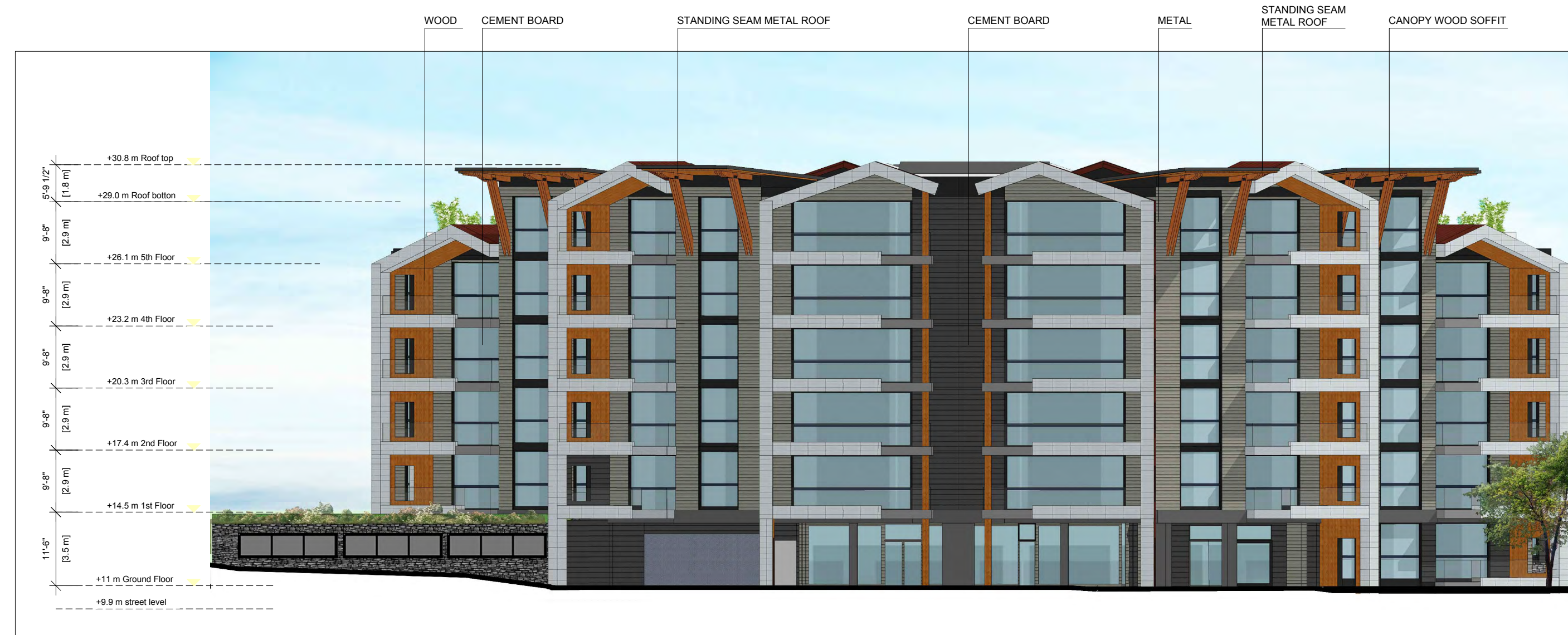
BUILDING B - NORTH EAST ELEVATION SCALE: 1:200
